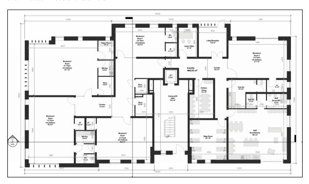
Figure 2.4 Proposed ground floor level of Block F illustrating layout of creche facility.
